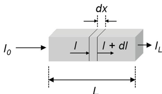
Figure 1 Attenuation of radiation intensity passing through the gas
