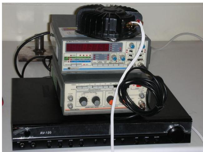
Fig. 3 - The vibration test equipment: on top the vertical vibration motor, underneath the frequency counter, frequency generator and at the bottom the audio amplifier.
