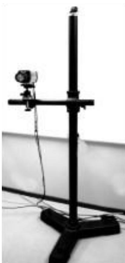
Fig. 5 - FLIR A40 IR camera on laboratory stand.
