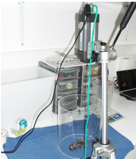
Fig. 3 - Thermal image acquisition setup and camera view.
