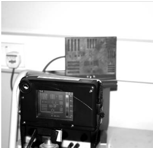
Fig.2 The IMPAC camera and heated resolution chart
