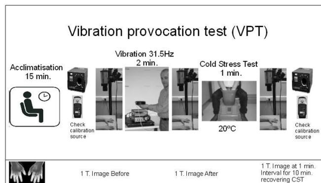
Fig. 6 - The Vibration Provocation Test (VPT) diagram.
