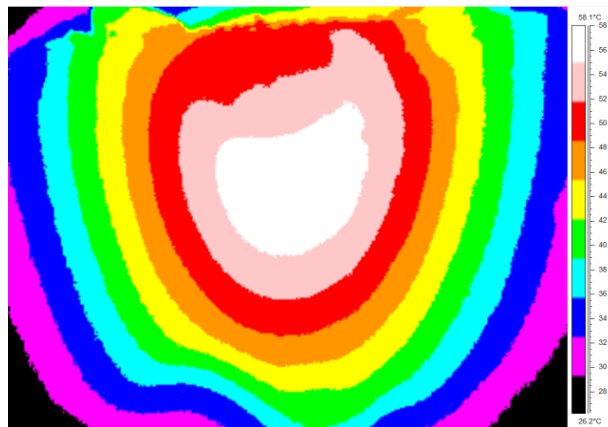
Fig. 3 - Temperature distribution at the end of drilling process.
