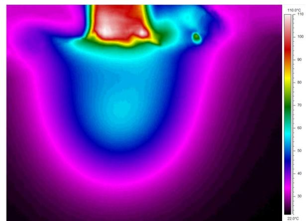
Fig. 2 - Hole drilling starting point, with close-up lenses.
