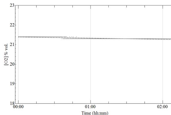
Fig. 5 - Linear regression analysis for O<sub>2</sub> concentration over a 2h trial at 30°C/90%HR with 2 people inside. (Legend: *Linear regression curve*: black dashed line; *Original data*: grey dots)
