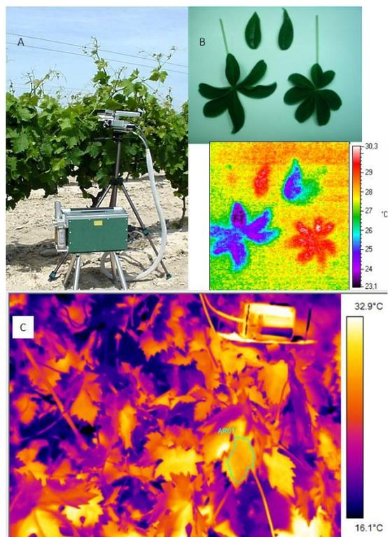
Fig. 1 - An infra-red gas analyser with a vine leaf inserted in the leaf chamber so as to measure stomatal conductance and other features of leaf gas exchange (A), digital (top) and thermal (bottom) images of lupin leaves, where the leaf on the right of the images is from a plant that had been subjected to drought, and the leaf on the left is from a plant that had been watered daily (B), and a thermal image of a section of grape-vine, showing a number of leaves (C).
