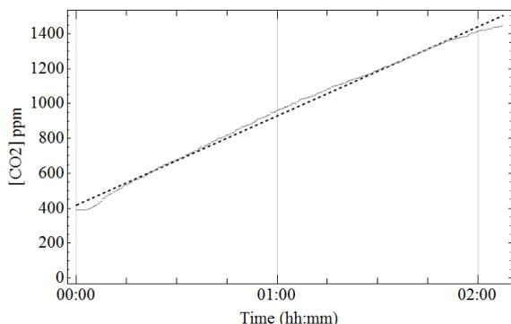
Fig. 4 - Linear regression analysis for CO<sub>2</sub> concentration over a 2h trial at 30°C/90%HR with 2 people inside. (Legend: *Linear regression curve*: black dashed line; *Original data*: grey dots)
